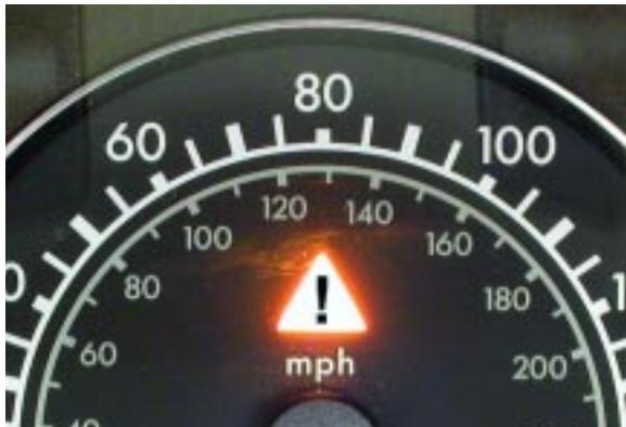
*The warning lamps come on as a bulb check when first starting. Then the warning triangle in the speedometer comes on to signal ASR activation. If the motorist toggles the snow-chain switch, the warning light stays on, flashing when wheelslip conditions occur.*
