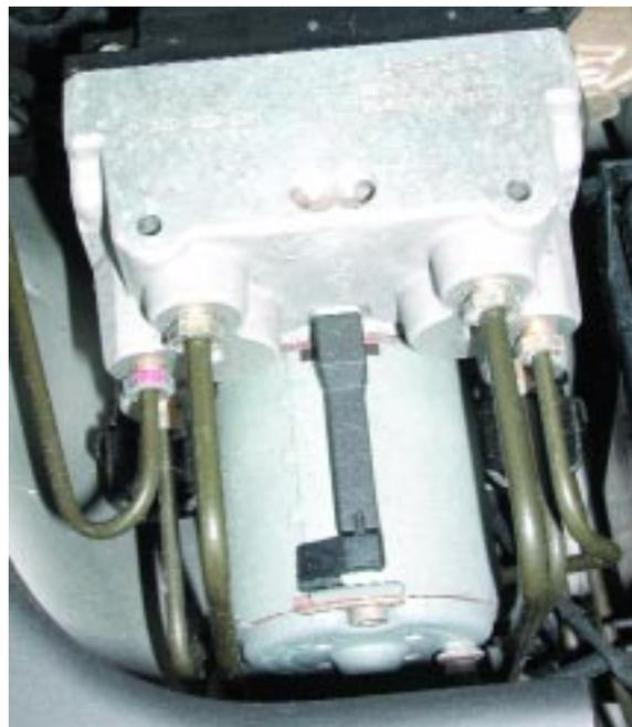
*All of the traction control systems employ electric motor pumps to build the brake fluid pressure required to activate the brakes during ASR activations.*
