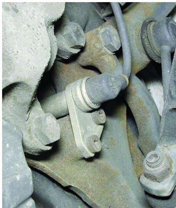
*All the traction-control systems function to begin with from the wheelspeed sensors input data. ASR uses sensors for both rear wheels, not just one at the differential, because it must identify which rear wheel slips to apply braking to the slipping wheel. The sensors are essentially the same inductive pickups used for all traction-control systems.*
